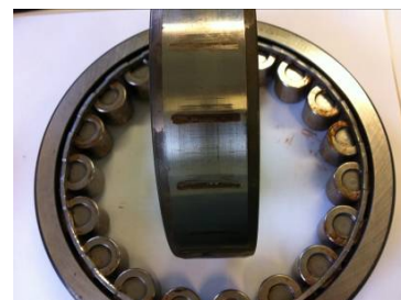
Figure 24: Surface marks (false brinelling)
