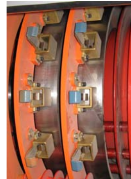
Figure 4: Brushes removed from the brush holder
