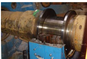
Figure 27: Corrosion on the shaft
