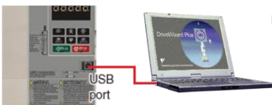
● Connecting L1000 and a PC with USB
