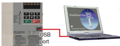
● Connecting L1000 and a PC with USB
