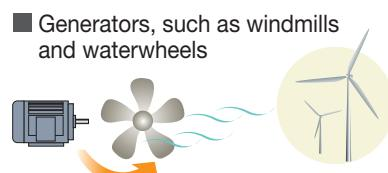
Wind, water, or another external force rotates a motor.
