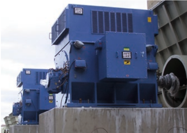
Supply: 9,900 HP, 13,200 V, 8 poles, IC01 Application: Fan
