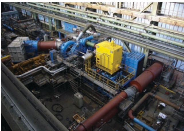
Supply: 14,000 kW, 10,000 V, 4 poles, IC86W Application: Test laboratory
