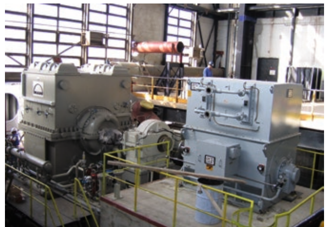
Supply: 12,000 kW, 6,000 V, 4 poles, IC81W Application: Centrifugal compressor
