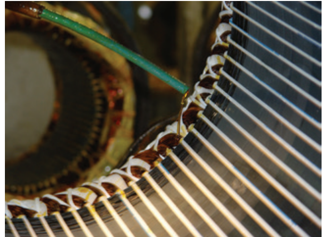
Figure 1.12.c - Resin applied by continuous flow process
