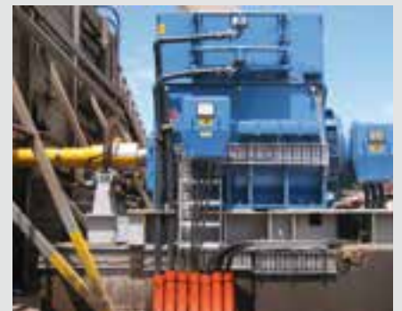
5,888 kW, 11,000 V, 14P, frame 1120 (MAW) SIMS METAL - Australia
