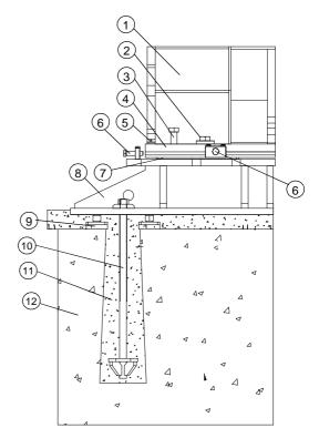
Figure 5.1: Example of anchor base installation
