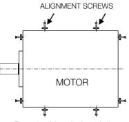
Figure 6.1: Motor horizontal alignment
