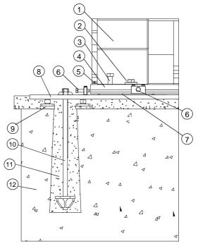
Figure 5.3: Example of soleplate installation
