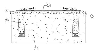
Figure 4.1: Example of foundation with fastening by soleplates
