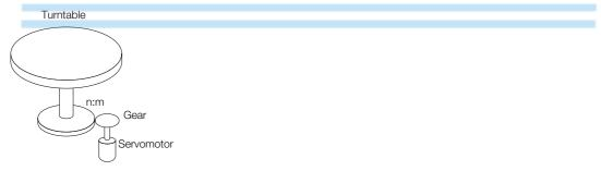
Because the turntable moves in only one direction, the upper limit to the number of rotations that can be counted by an absolute encoder will eventually be exceeded.
