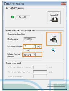
When measurements have been completed, the measurement results will be displayed.
