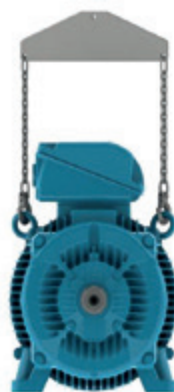
Figure 4.6 - Use of a spreader beam for lifting
